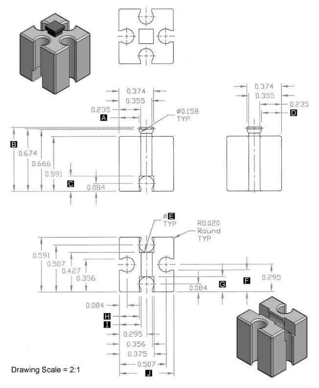
Study the technical drawing of the fischertechniks® building block. Ten of the measurements/dimensions (A through J) have been omitted from the drawing. You will use the dial caliper to measure the actual block and find the missing dimensions to the nearest .001 inch.
